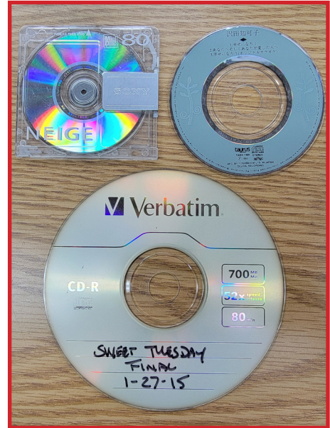
Mini disc (top left), mini compact disc (top right) and compact disc (bottom).
